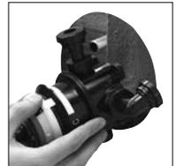
**10** Using a silicone based lubricant, lubricate the supply pipe ends and whilst supporting the elbows, push home the supply pipes ensuring the correct orientation for the inlet pipes (HOT LEFT AND COLD RIGHT AS SHOWN ON THE VALVE BODY). Push the valve fully home until a definite stop is reached (tube insertion depth is 25mm). Secure the valve assembly to the fixing surface using the screws provided.
