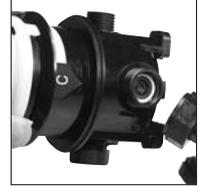
**8** The Colt valve is supplied with an outlet cap on the bottom of the valve allowing for a top outlet connection. The bottom outlet can be used by simply removing the cap and repositioning it on the top outlet. If the cap is removed please ensure that when replaced the membrane in the cap is in place and that the cap is done up tight.
