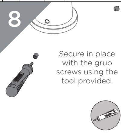
Secure in place with the grub screws using the tool provided.
