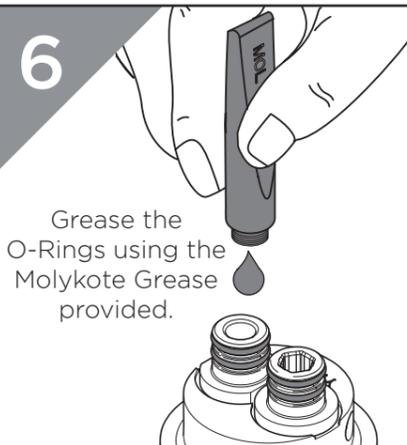
Grease the O-Rings using the Molykote Grease provided.
