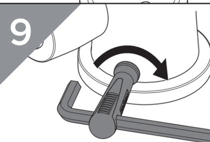
Thread the hexagonal key through the EasyFit tool and tighten the grub screws with an extra 1/2 turn.
