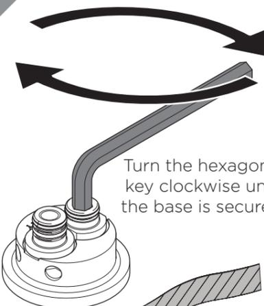
Turn the hexagonal key clockwise until the base is secured.
