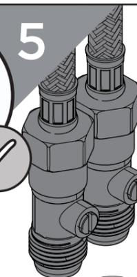
Connect the hot and cold water connections.
