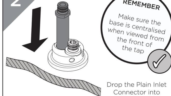
Drop the Plain Inlet Connector into the base.
