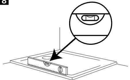
Place shower tray **A** onto the wet cement ensuring that it is fully supported. Check the level of the top rims only as the shower tray has built-in fall for adequate drainage.
