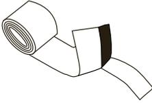
Wipe the surfaces clean where the strip will be attached first with a clean damp cloth, allow to dry and then wipe with the IPA wipe supplied in the kit.
