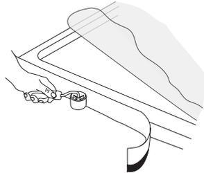
**Note!** Some shower trays have a protective film (indicated by a label on the surface) which **MUST** now be removed. Undertake a final inspection of the shower tray at this stage. **DO NOT PROCEED IF NOT SATISFIED.**
