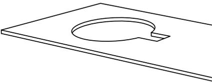
**Note!** With some types of waste unit, it may be necessary to form a keyhole shaped cut-out in the ply using a jigsaw. This will make access to the waste unit easier.
