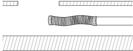
Remove the plywood and install the waste outlet pipe in the cavity in accordance with building regulations.
