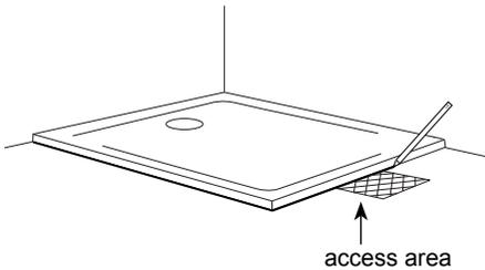
Place the shower tray **A** in position on the floor (ensuring surface is level) and mark the perimeter and waste hole on the floor including an area outside the perimeter for access to connect plumbing (as dictated by the installation location) after the shower tray has been installed. If using a shower tray with a built in tiling upstand, allowance must be made for recessing the tray into adjacent walls to allow tiling down onto the tray surface.
