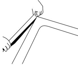
Attach to the edge of the shower tray so that it is square and the edge protrudes at least 20mm above the edge of the tray.
