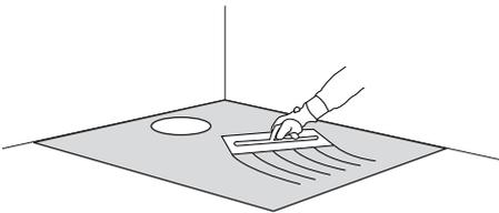
Mix fine sand, cement and a cement additive in accordance with the manufacturers instructions to a workable mix to cover the total area under the tray. Trowel to a thickness suitable to allow leveling and full support of the shower tray.
