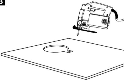
**Note!** With some types of waste unit, it may be necessary to form a keyhole shaped cut-out in the ply using a jigsaw. This will make access to the waste unit easier.
