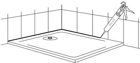
When the cement has set, make connection between the shower tray and waste piping. The shower tray and all connections **MUST** now be checked for water tightness, flow and adequate drainage over the entire area.
