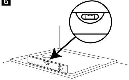
Place shower tray **A** onto the wet cement ensuring that it is fully supported. Check the level of the top rims only as the shower tray has built-in fall for adequate drainage.
