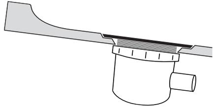
Fit the waste unit to the shower tray following the instructions supplied with the unit and protect exposed threads with masking tape. Before proceeding dry fit all items in-situ to ensure compatibility and then screw the plywood level into position.
