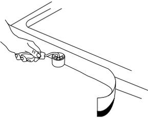
Using a small roller or other appropriate tool roll the seal strip so that it attaches firmly to the edge of the tray removing any bubbles or creases, paying particular attention to the corners.
