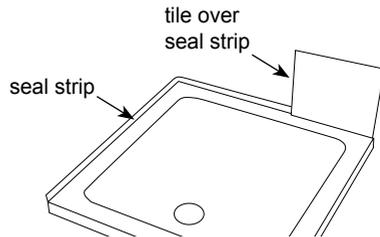
Install the shower tray in the correct position and tile in front of the seal strip.
