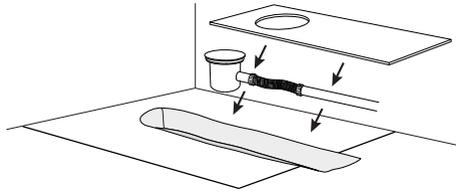
Form a trench in the floor to hold the waste unit and piping.
