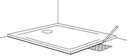
Place the shower tray **A** in position on the floor (ensuring surface is level) and mark the perimeter on the floor including an area outside the perimeter for access to connect plumbing (as dictated by the installation location) after the shower tray has been installed.
