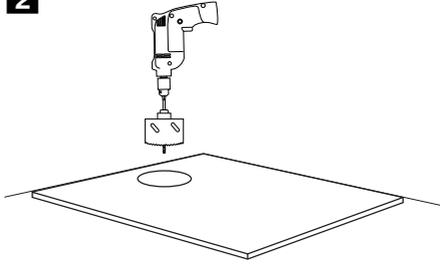
The floor area (or larger) covered by the shower tray must be removed and replaced with a single level piece of plywood (minimum 18mm thick).
