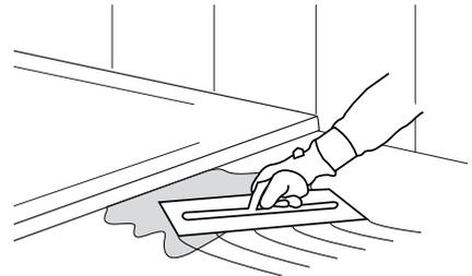
Fill in the access area and the waste pipe trench beneath the shower tray **A** with cement to give full support to the shower tray when in service.
