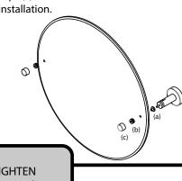
If necessary tighten or loosen the mirro r's tilt mechanism by using a flat head screwdrive r.
