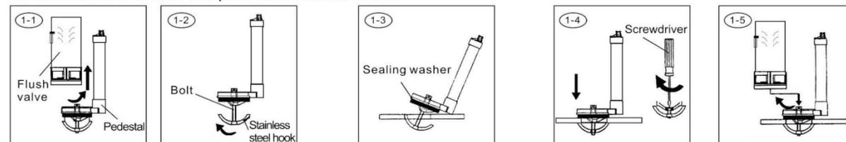
Contrarotate drainage body and make it removed from pedestal.
