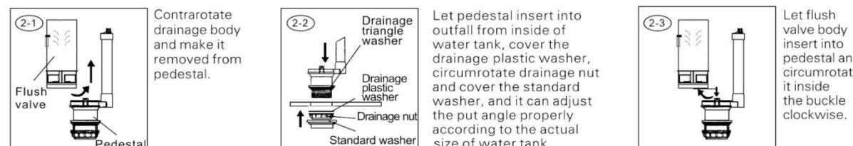
Contrarotate drainage body and make it removed from pedestal.
