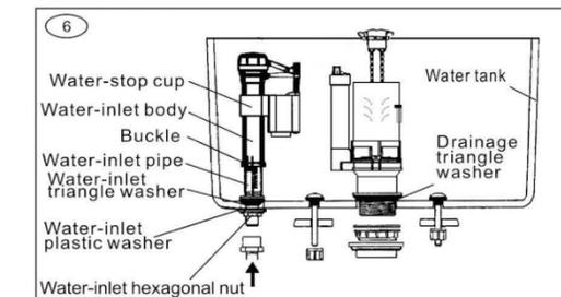
As photo show, connect water-inlet pipe to test and notice the following phenomenon:
