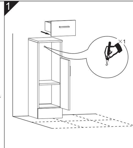
please drill the holes according to the hole position mark on the wall
