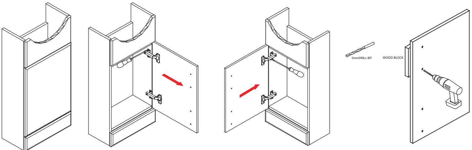
Floor Standing units must be fitted back to the wall through the backrail using suitable fixings. (not supplied)
