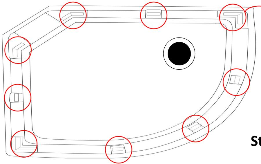
Apply RubberGum to raised sections of the tray and remove backing paper.
