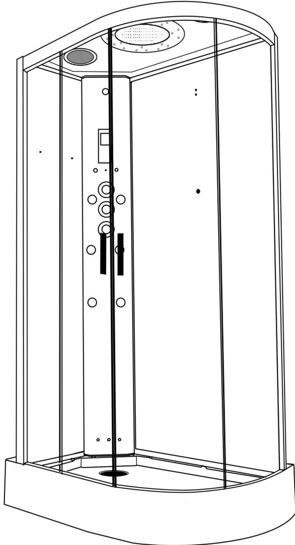
1. Please ensure all the connections are watertight including the waste, body jets, internal and external hoses and steam connections (model dependent).
