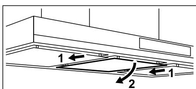
2. Slightly tilt the front of the filter downwards, then pull.
