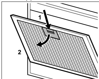
3. Slightly tilt the front of the filter downwards (2), then pull. Repeat the first two steps for all filters.
