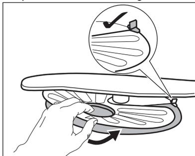
7. Reassemble the filters (B) and (C).
