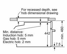
If the compact appliance will be installed underneath a hob, the following worktop thicknesses (including substructure if necessary) must be taken into account.
