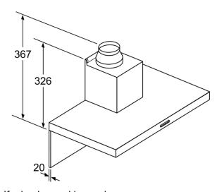
If a back panel is used, the design of the appliance must be considered. measurements in mm
