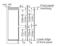
The specified unit door dimensions are valid for a door gap of 4 mm.
