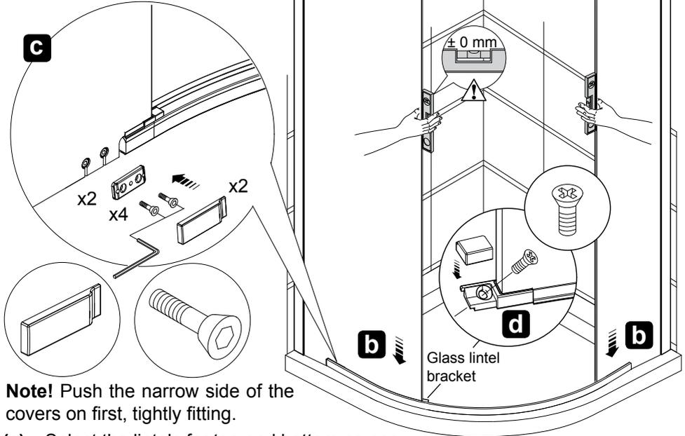
**Note!** Push the narrow side of the covers on first, tightly fitting.
