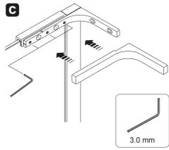
**Note!** Ensure that bracket is not overtightened onto tiles to ensure cover can still slide into notch.
