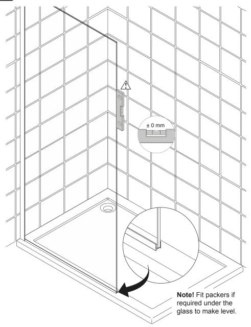
(a) Make sure that the glass panel is level and the H-Section is equidistant from the edge of the tray.
