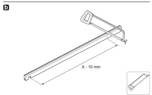
(a) Cut the bracing bar to the measured dimension 'X' minus 10 mm (X - 10 mm). e.g. If the measured dimension is 760 mm then cut the bracing bar to 750 mm
