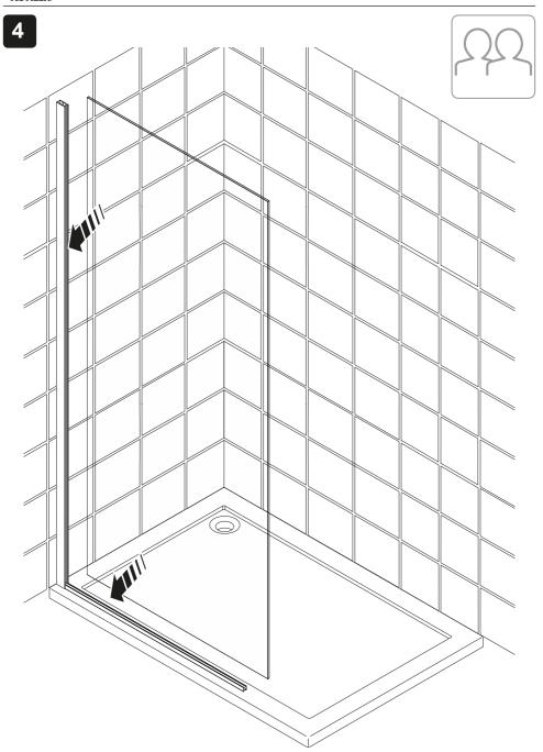
(a) Install the glass panel into the wall channel that had been secured to the wall earlier. Ensure that the glass is fitted level with the end of the H-Section.
