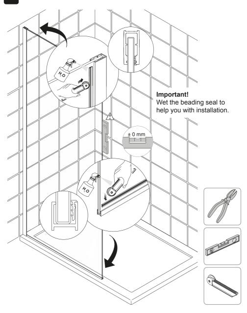
(a) Push in the beading seals using the roller provided on the wall channel and H-section. Trim the beading seal 15 mm from the top of the glass.
