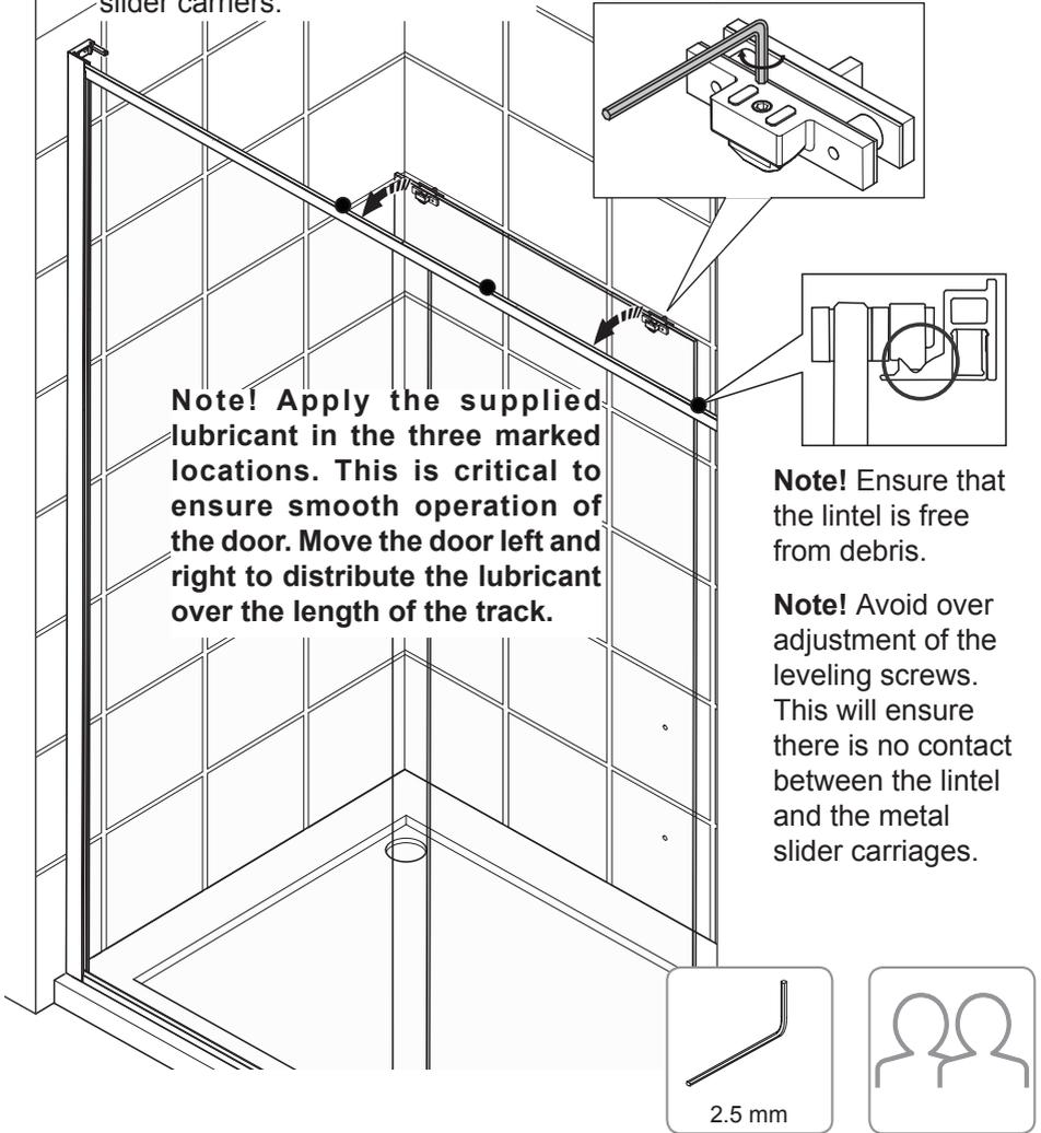
**Note!** Apply the supplied lubricant in the three marked locations. This is critical to ensure smooth operation of the door. Move the door left and right to distribute the lubricant over the length of the track.
