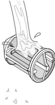
Rinse each filter in clean warm water, removing any dirt or debris. Replace if the filter mesh is damaged. Make sure both filters are refitted correctly into the elbows.
