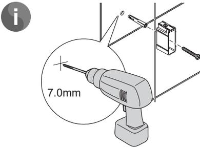
Drill the fixing hole for the top support and fit the wall plug and screw top support into position.
