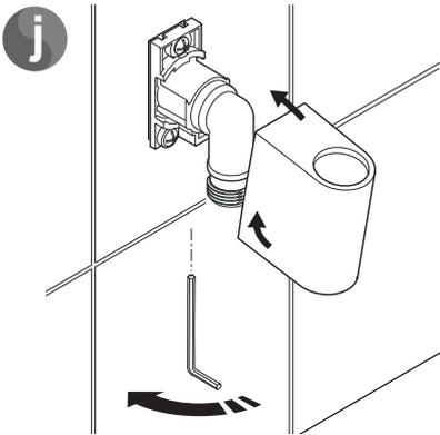
Fit the cover over the elbow and lock into place by turning the grub screw anticlockwise.
