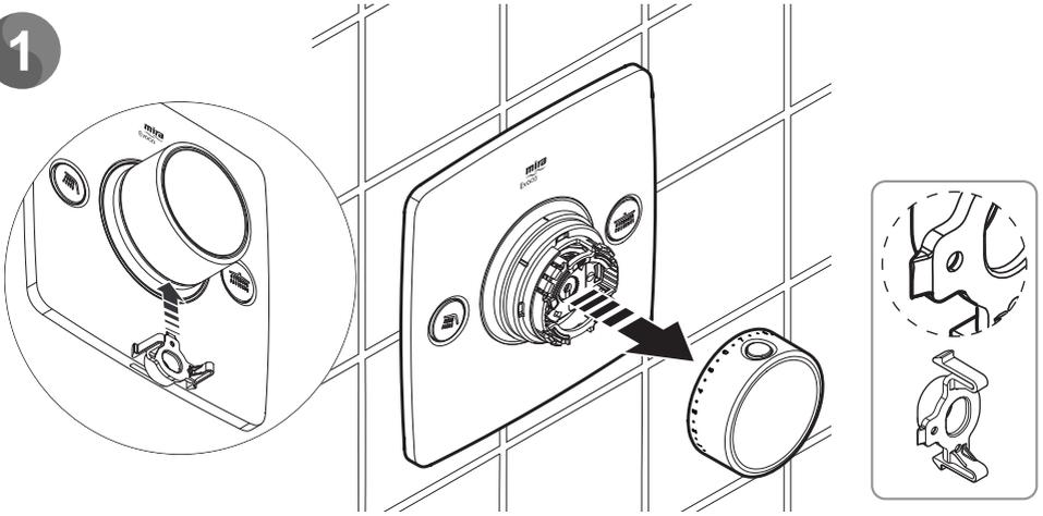
Remove the handle by using the blade on the setting piece, place in between the bottom of the handle and shroud and twist to unclip the handle.
