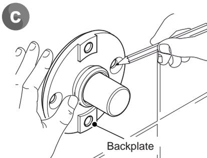
Mark the positions of the backplate fixing holes.
