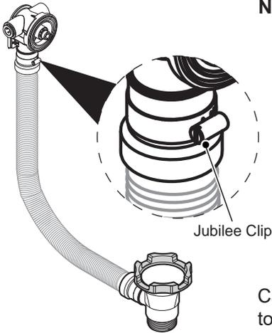
**Note:** When the bath filler waste is extended, there may be a need to rotate the bodies to allow alignment to the both mating surface.
