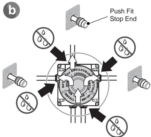
Isolate the water supply and fit the push fit stop ends (not supplied) to the outlets. Re-open the water supply and check for leaks.
