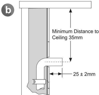
The outlet pipe must protrude 25mm ( $\pm 2$ mm) from the finished wall surface.
