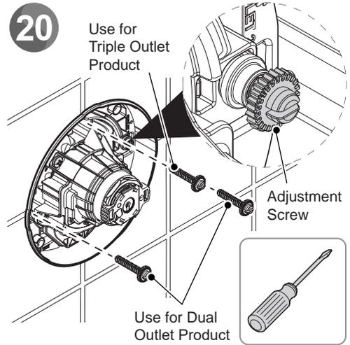
Attach two or three adjustment screw depending if installing a dual or triple outlet product by screwing into the respective slot using screwdriver.
