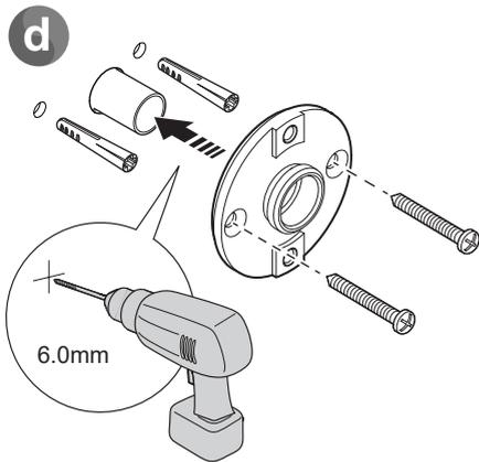
For solid walls drill the fixing holes for the backplate with a 6mm drill and insert the wall plugs (supplied). For other types of wall structure alternative fixings may be required (not supplied).
