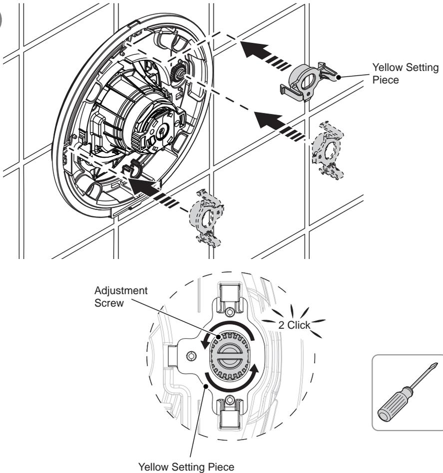
The adjustment screws have to be set to ensure when the concealing plate is fitted the on/off buttons work correctly to turn the shower on and off.
