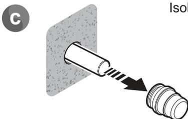
Isolate the water and remove the caps.
