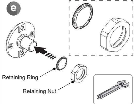
Place the retaining ring and nut over the pipe in the orientation shown and tighten in place using suitable size wrench. **DO NOT** overtighten.
