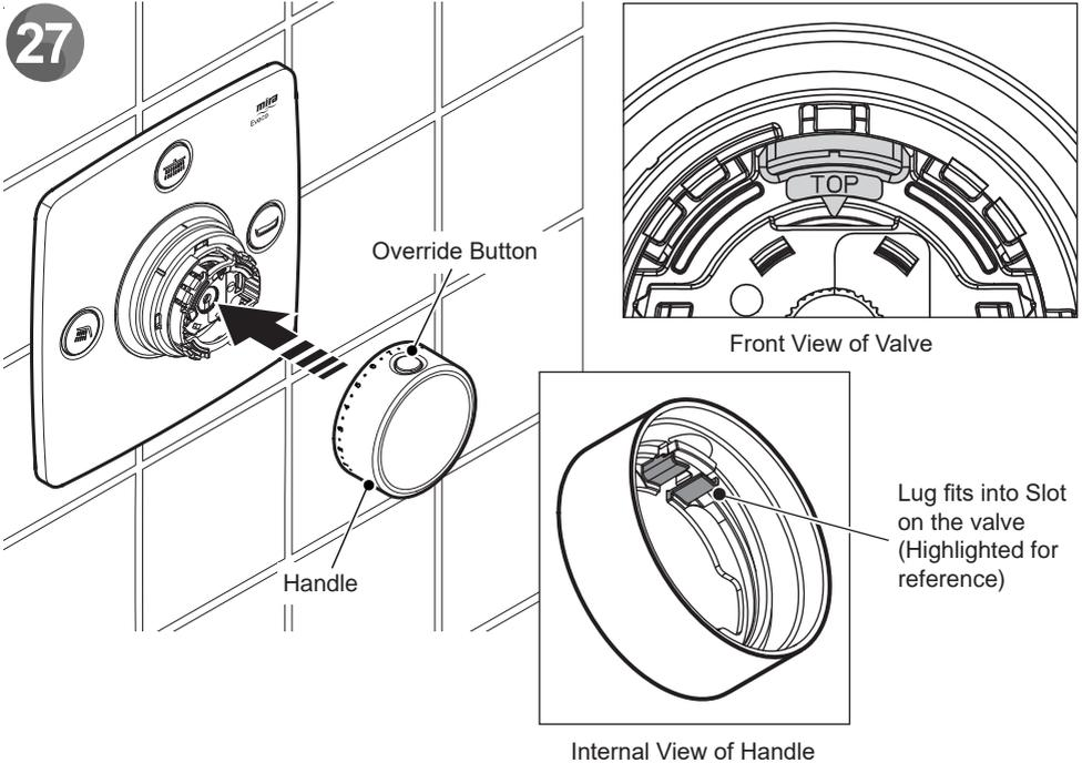
Push fit the handle ensuring that the override button is set at 12 O'clock position and the lug on the inside of the handle matches up with the slot available on the valve.
