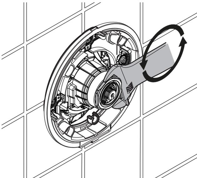
Carefully loosen the hexagonal head nut as shown.
