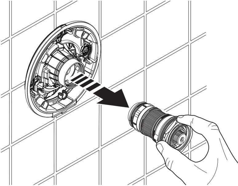
Carefully pull out the cartridge from the mixing valve.
