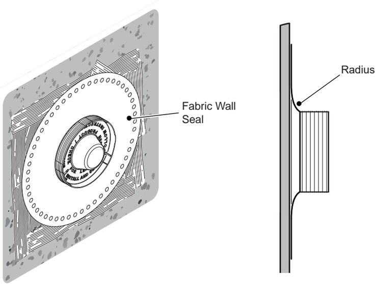
Fit the fabric wall seal and press flat around the edges, creating a radius around the sides of the Building in Box.
