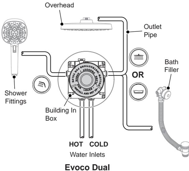
Fit the outlet pipework ready for connection to either a right angle connector for a handset, bath (adjustable fitting), or a shower arm for a fixed spray head (rigid fitting).
