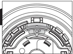
Front View of Shroud installed on Valve
