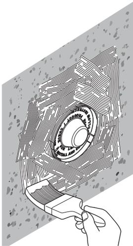
Apply further adhesive over the fabric wall seal and around the sides of the Building in Box.
