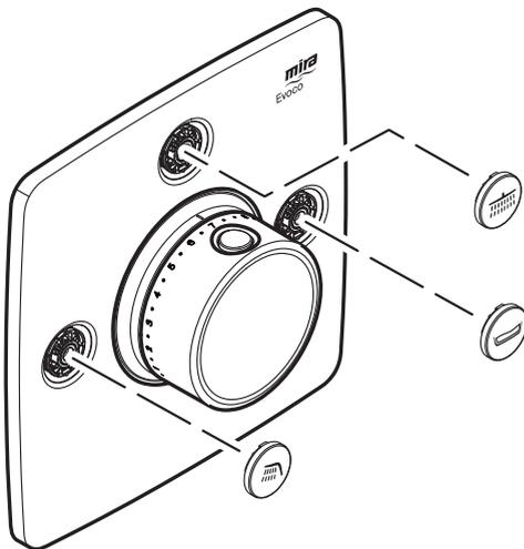
The button graphics come in set positions, if this is not suitable for your installation, use the button cap removal tool to remove the cap and swap the caps over.
