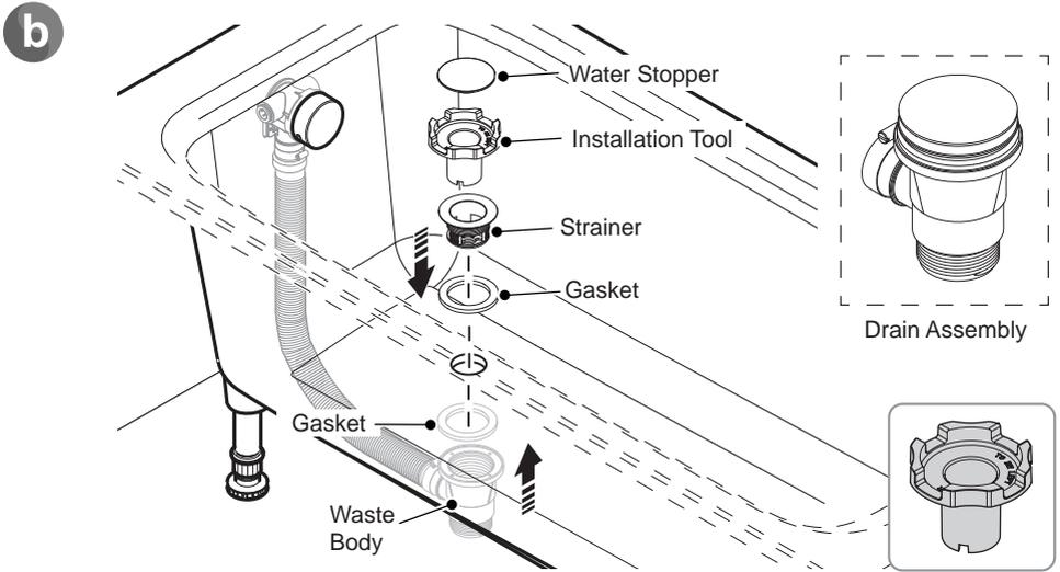
**Note:** An installation tool is supplied, this is stowed within the assembled waste body for packing purposes. Use this tool to screw the strainer into the waste body.
