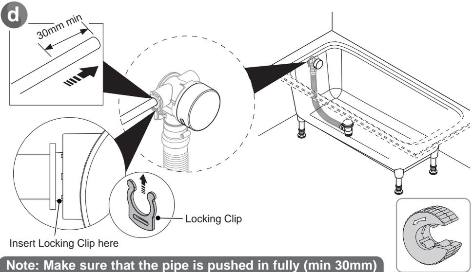
**Note:** Make sure that the pipe is pushed in fully (min 30mm) until it hits the internal stop feature.
