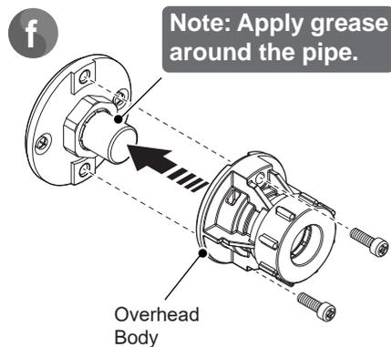
Fit the overhead body over the pipe and secure with the fixing screws provided.
