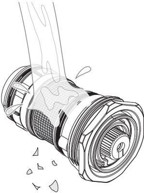
Rinse the filter in clean warm water, removing any dirt or debris.
