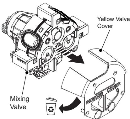
Remove the cover from mixing valve.
