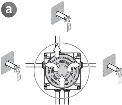
Turn on the water supply and flush the outlets.
