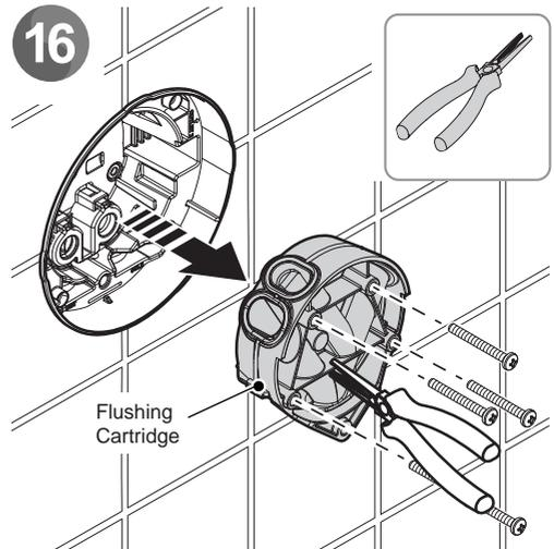
Make sure both water supplies are isolated before removing the flushing cartridge.
