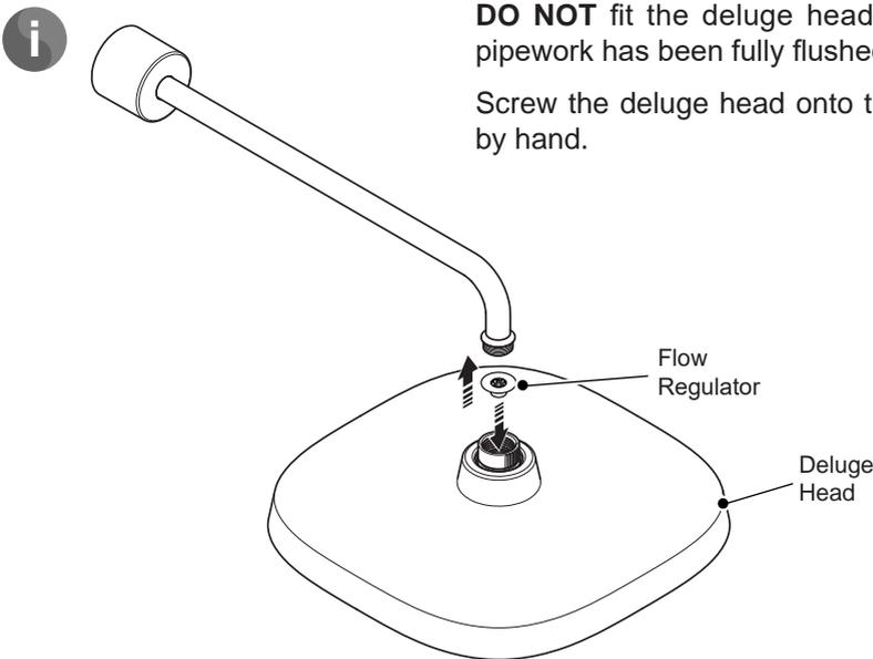
**DO NOT** fit the deluge head until after the pipework has been fully flushed through.
