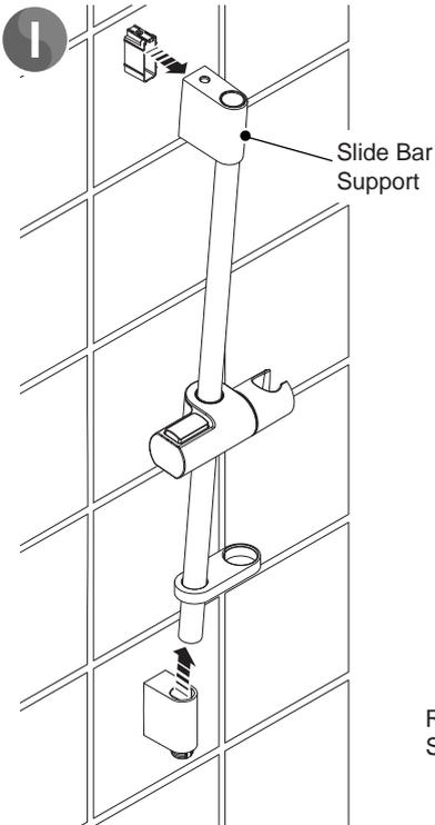
Carefully remove the slide bar assembly and tighten the screw on the back of the slide bar support to secure in position.
