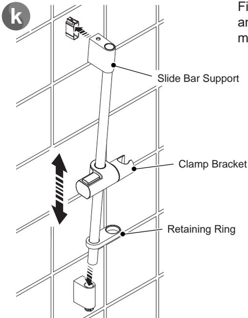
Fit all the components onto the slide bar and fit the slide bar assembly in position, making sure that it locates correctly.
