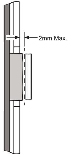
Taking care to prevent damage to the wall finish, trim the Building in Box back to within 2 mm from the finished wall surface.
