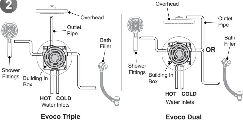
Determine the pipework route. All pipework to the product must be clipped and supported to prevent movement and pipe noise due to any pulse pressures.
