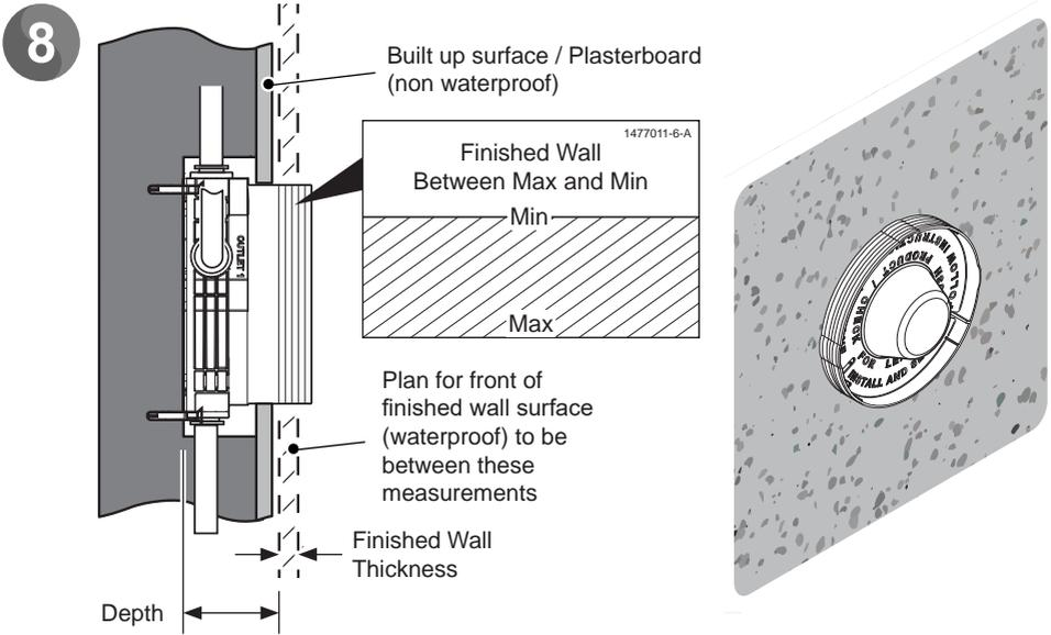
**Note:** Refer to details of cavity depth and finished wall thickness.
