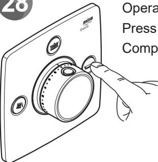
**Note:** If outlet does not turn off or insufficient water flows from the product, refer to commissioning to remove the handle and shroud and re-set the adjustment screw height following installation step 23 & 24.
