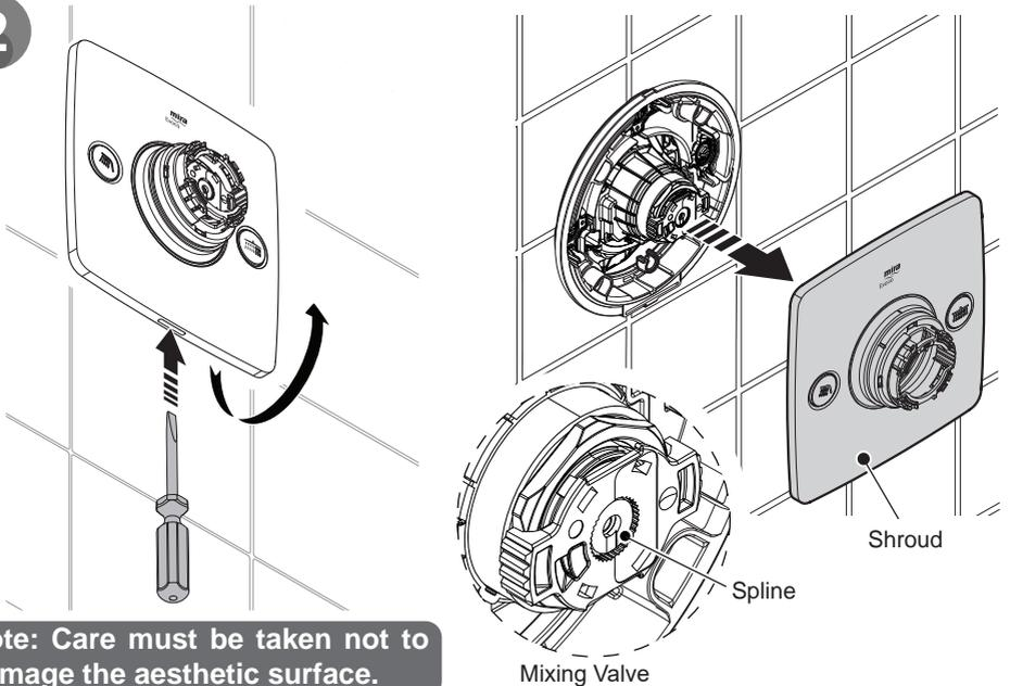
**Note:** Care must be taken not to damage the aesthetic surface.
