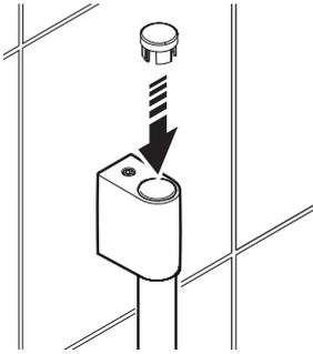
Fit the cap to the top of the slide bar.
