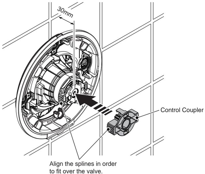
**Note:** Fix the control coupler if the front of the mixing valve is less than 30mm from tile.
