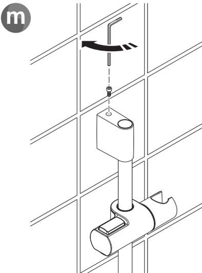
Secure the assembly in position with the screws. The top securing screw tightens **Clockwise**, the bottom one **Anti-clockwise**. **Do not overtighten!**
