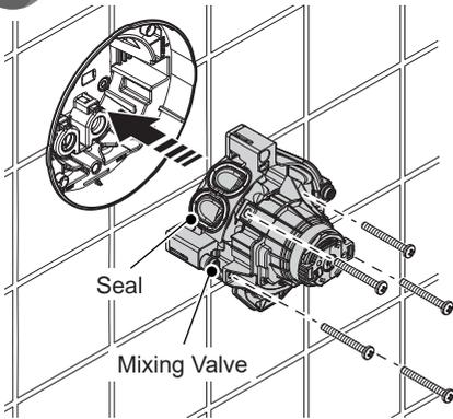
Push in and fully secure the mixing valve into the Building in Box using the provided screws that were removed on step 16. **DO NOT** use a power driver.
