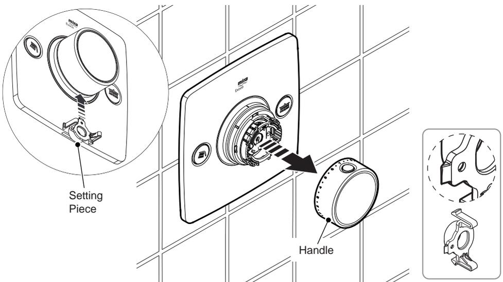
5. Remove the maximum temperature peg from the top of the valve by using a screwdriver. Refit the handle.
