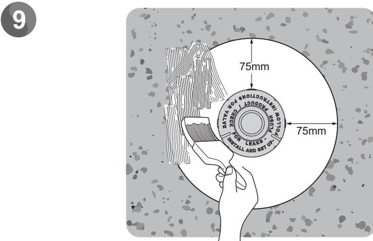
Apply a liberal coat of waterproof adhesive (not supplied) around the product. Use a suitable waterproof shower tanking adhesive. We recommend a liquid based plumbing type to be applied with a paint brush, available from tile/builder merchants. A sufficient amount is required for coating this area twice during the installation.
