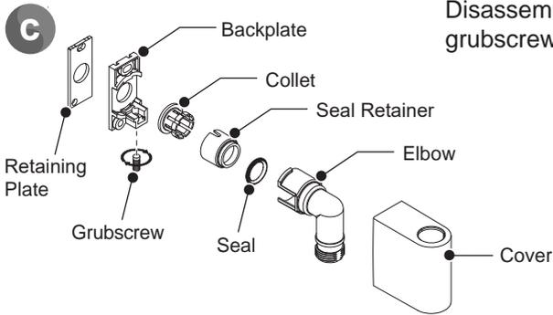
Disassemble the components by turning grubscrew clockwise.
