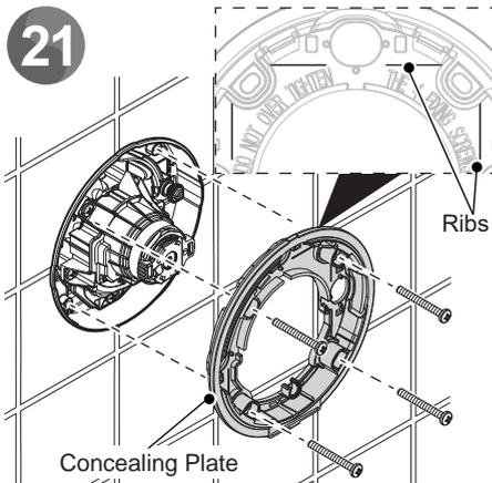
Align ribs on concealing plate parallel to the tiles and secure the concealing plate using the four screws provided in component pack.
