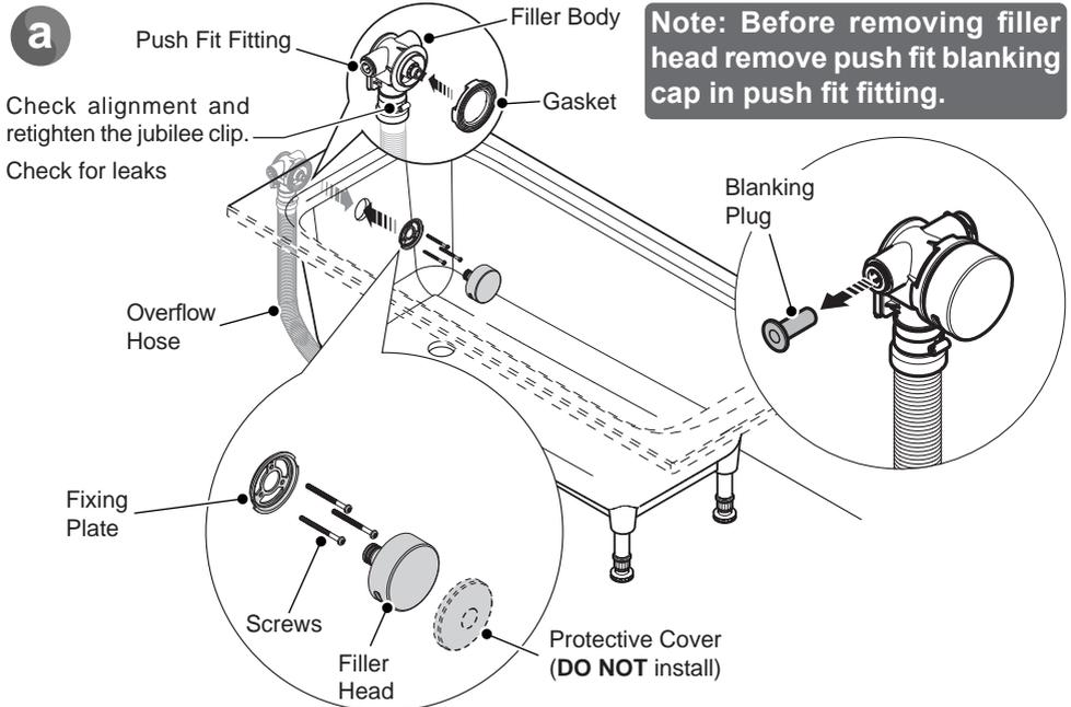
**Note:** Ensure the screws are not cross threaded and are tightened evenly. Hand tighten only. **DO NOT** use a power driver to tighten the screws. Important! When installing the Mixer Valve to be used as a bath filler ensure the flow rate of the bath overflow fitted exceeds the flow rate output from the Mixer Valve.
