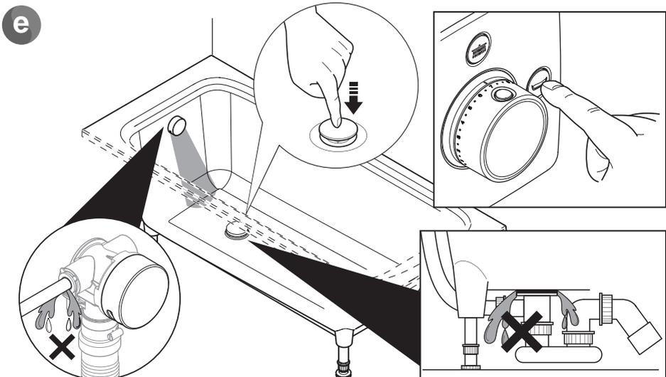
Turn on the water supply and check for leaks from the waste and the bath filler connections.
