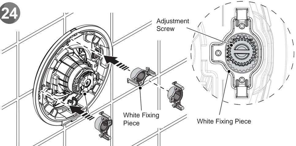
Place the fixing piece over the adjustment screw (as shown). Push and clip the fixing piece to lock adjustment screw in position.
