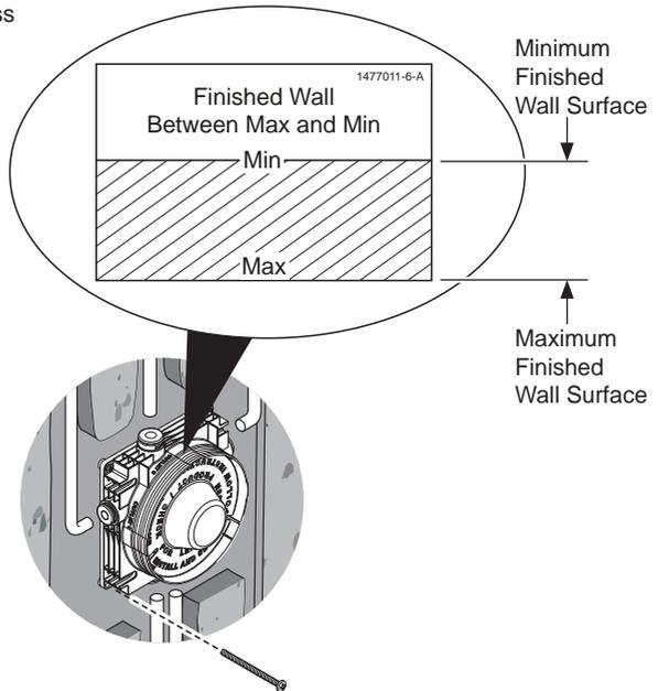
Create a suitable cavity for the Building In Box and the pipework.
