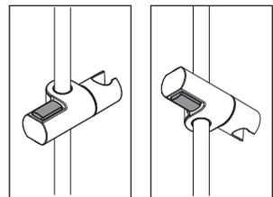
**Important! Press the buttons on the clamp bracket to slide it through the slide bar.**
