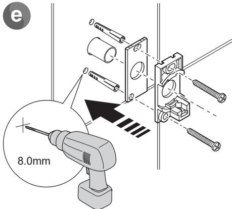
The screws and wall plugs supplied are suitable for most solid wall installations. Alternative fixing screws for panel structures are not supplied.
