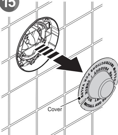
Remove the cover but do not throw away as it can still be used to stop debris during finishing of the installation.
