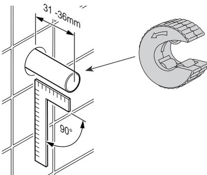
The right angle connector must be fitted to a waterproof, flat and even wall surface.
