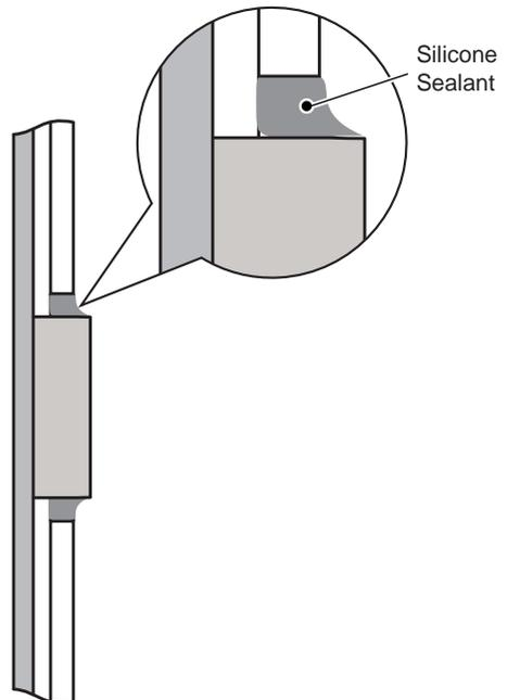
Apply silicone sealant to fill the gap around the Building in Box.
