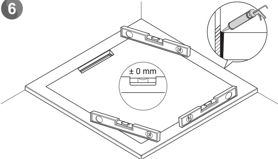
Place the shower tray on your base (sand/cement or silicon) and using a spirit level check that it is straight and level.
