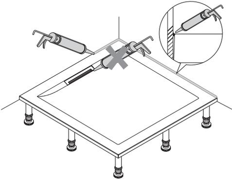
Seal the legs to the floor with silicone sealant. Apply silicone sealant to the locknuts to secure in position. Apply silicone sealant in accordance with the manufacturer's instructions to seal the shower tray to the wall.
