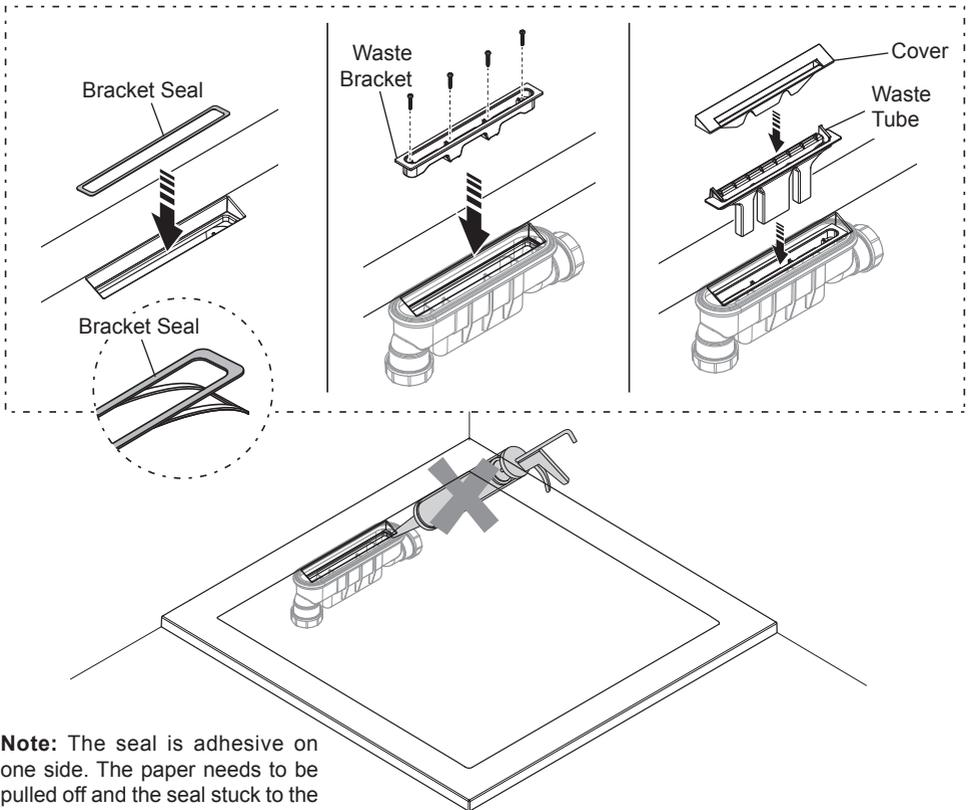
**Note:** The seal is adhesive on one side. The paper needs to be pulled off and the seal stuck to the underside of the tray.
