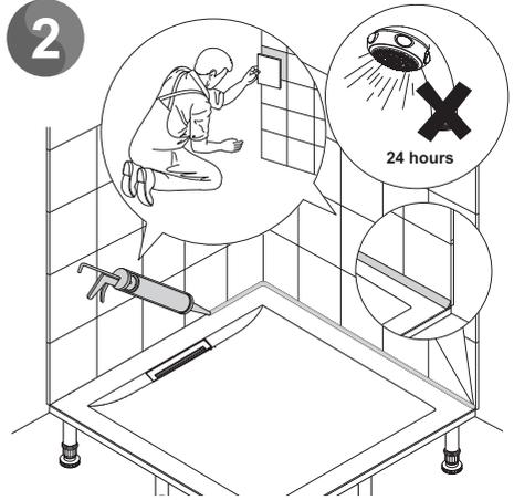
Tile the walls down on top of shower tray. Apply silicone sealant in accordance with the manufacturer's instructions to seal the shower tray to the tiled wall surface.
