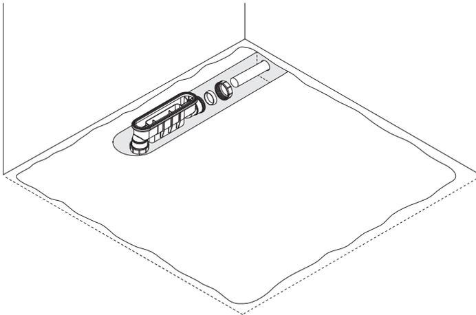
For water to drain away properly, the waste pipe must have a fall of at least 3cm per meter. The waste pipe must be properly supported to hold its own weight and that of the waste assembly.
