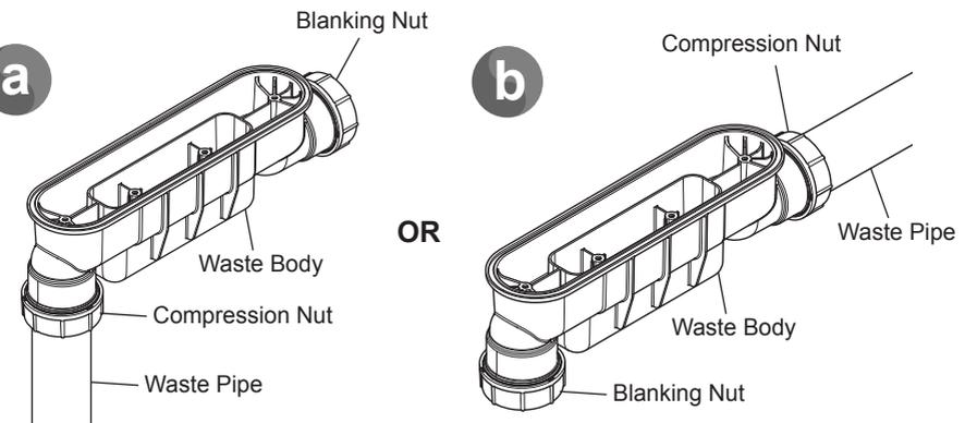
The waste has two drain outlet options. Utilise the outlet suitable for your waste pipe configuration.
