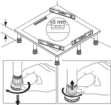
Place the shower tray on a flat surface and using a spirit level check that it is straight and flat and that the shower cubicle will sit on its surface correctly when fitted. Make sure locking nuts are secure.
