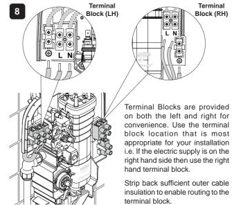
Ensure the earth bonding complies with relevant regulations. (Live) = Brown wire (\frac{1}{2}) (Protective Earth) =
