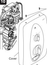
aligned with the spindles and replace the cover. Tighten the three cover
