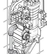
pipe to the inlet connector using a push fit elbow or an elbow with compression nuts and olives. Turn on the water supply
