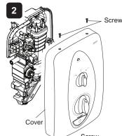
From the new shower, remove the three screws that hold the cover on then remove the cover.
