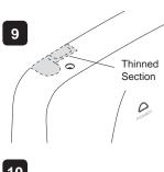
For falling or rising supplies the cover has thinned sections on the top and bottom that can be removed to allow entry of the supply pipe and electrical cables
