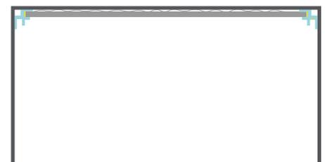
Push panel into internal corner and press against wall firmly, clean any excess silicone from corner.
