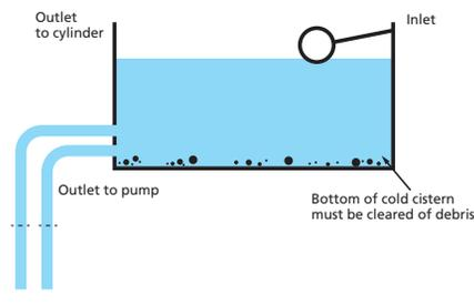
In systems with more than two bathrooms, the cold water supply to the cylinder must be in 28mm pipework.
