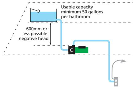
Tank fed, pressurised cylinder or combination boiler system with single-ended Right Universal pump to boost the hot supply water pressure and cold water mains supplies 'cold' to shower, bath, basin and toilet.
