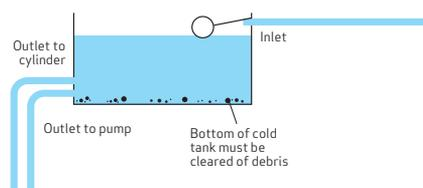
Multiple cold water storage tanks **MUST** be linked in 28mm pipe work with the bottoms of the tanks at the same level.
