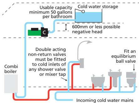
Tank fed (hot) with cold water mains systems **MUST** use Right pump universal.
