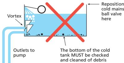
Chronic aeration of the pump occurs when this problem is combined with inadequate storage capacity and/or when the volume of water drawn by the pump and other services exceeds the refill rate and creates a vortex which draws air and possibly debris into the pump.
