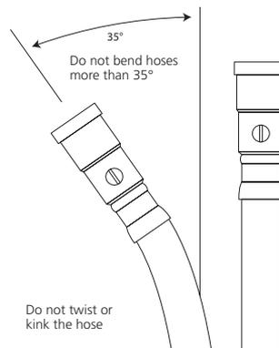
Ideally the AV couplers should be straight, but they must **NOT** be twisted or bent more than 35° (this invalidates the warranty). See Figure 5 above.
