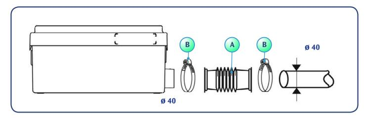
Use the rubber connector (A) for connection of pipes to the side inlets. Secure with the metal hose clips (G).
