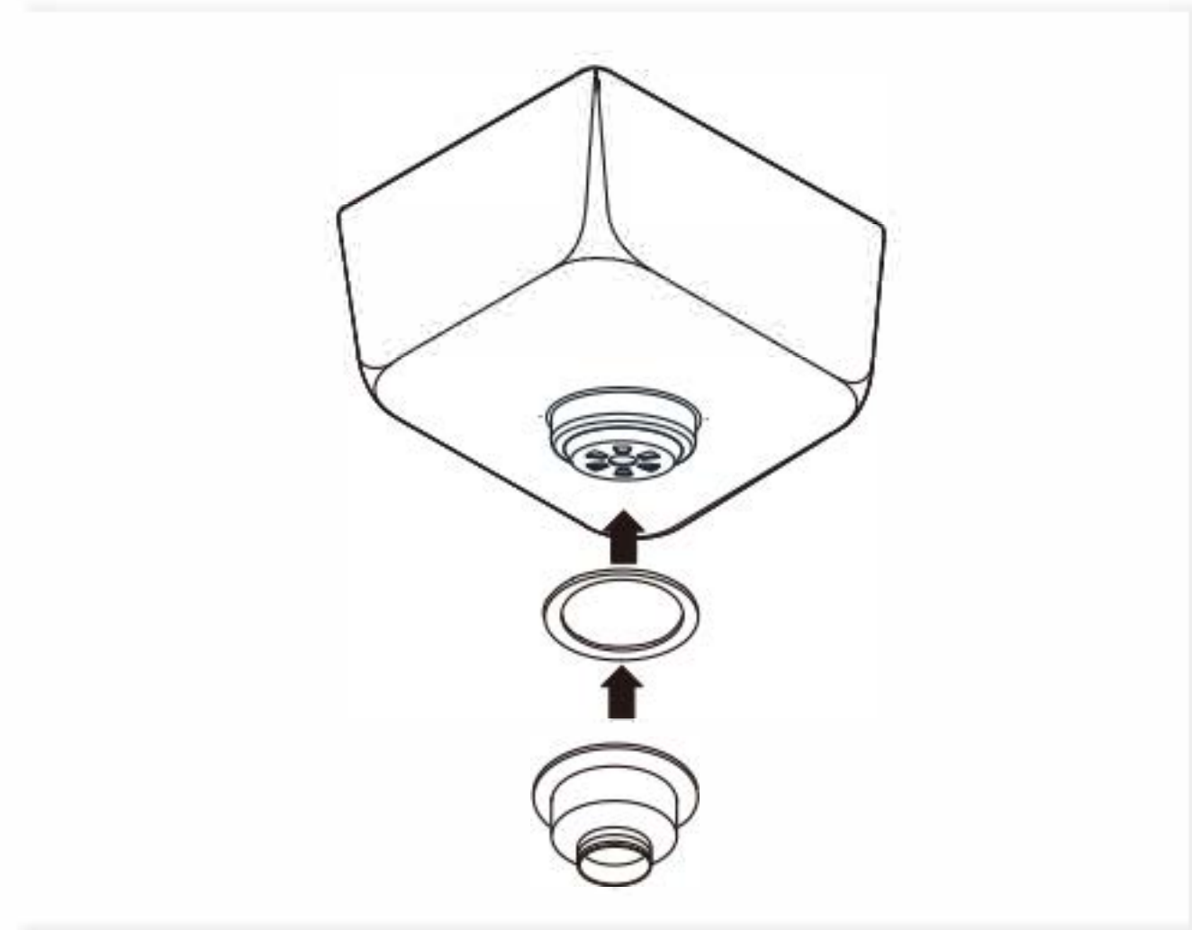
Step2: Put the lower strainer and black gasket connect to the upper part under the sink.
