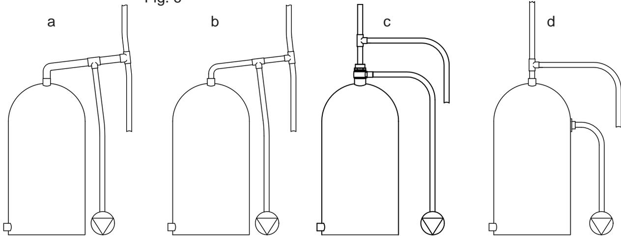
Off expansion pipe with rising 28 mm offset reducing to 22 mm pipework to pump and expansion pipe.
