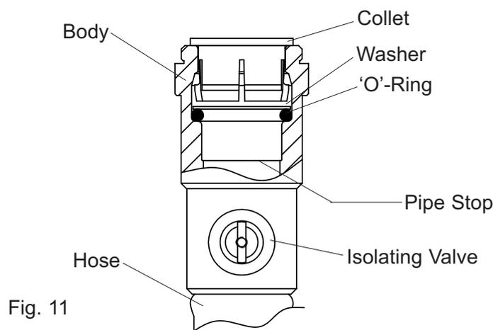
4. Push pipe firmly into fitting, until pencil mark is level with the top of the collet and the pipe stop resistance is felt. Pull on pipe to check it is secure and correctly fitted.
