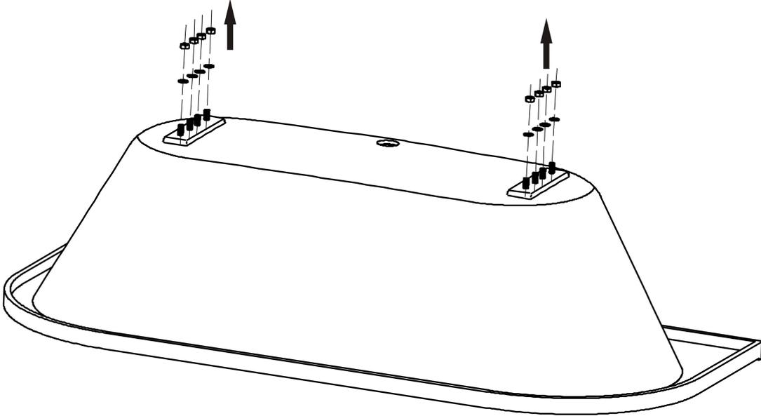
**2** Attach the brackets to the base of the bath and secure with nuts, washers and backup rings supplied with bath.
