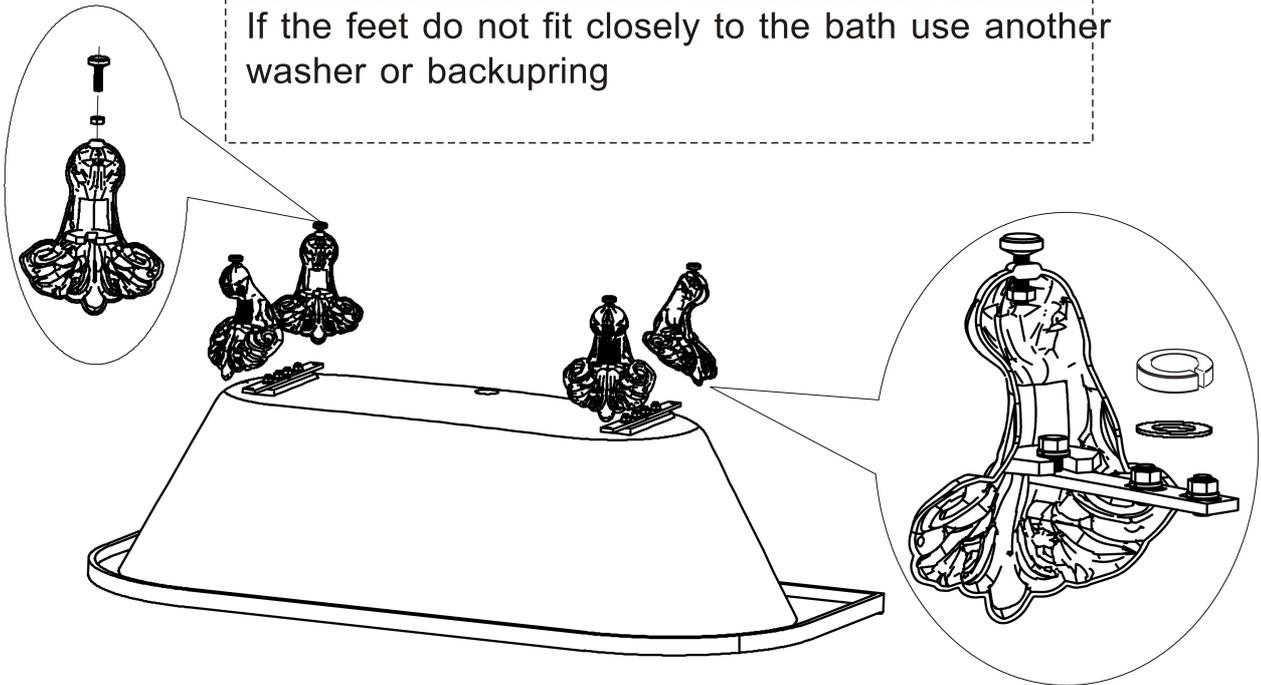
**4** Turn the bath over and level using the feet adjusters.
