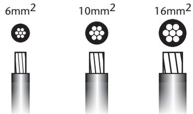
1. Measure the width of an individual strand, and half that measurement to find  $(r)$ , e.g:  $1.34\text{mm} \div 2 = (r) 0.67\text{mm}$
