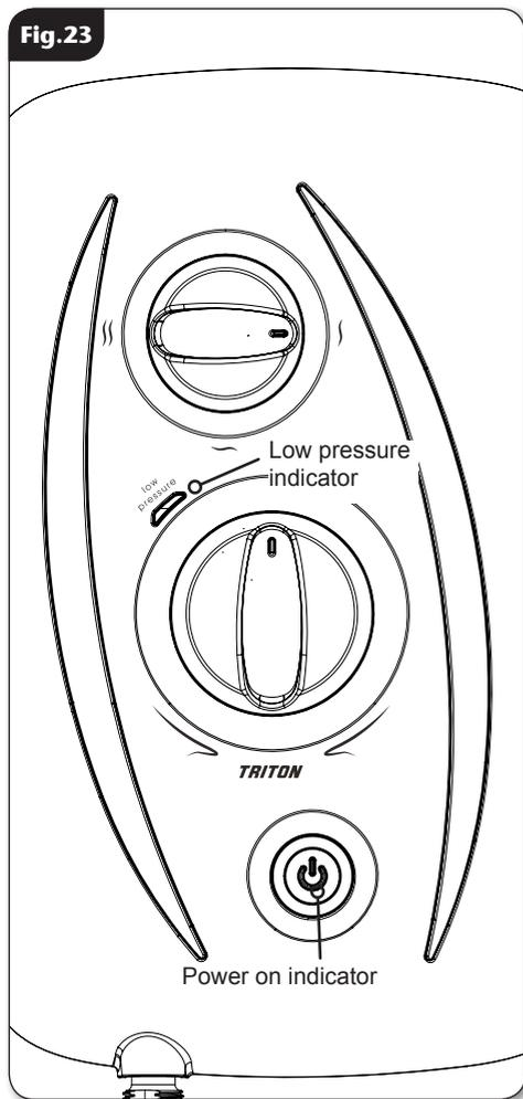
**NOTE:** In normal use, it is in order to leave the water supply permanently on to the shower unit, but as with most electrical appliances, **the unit MUST be switched off at the isolating switch when not in use.**
