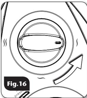
**D.** With the cover off the shower - turn the temperature control fully clockwise to the 5 o'clock position (**fig.17**).
